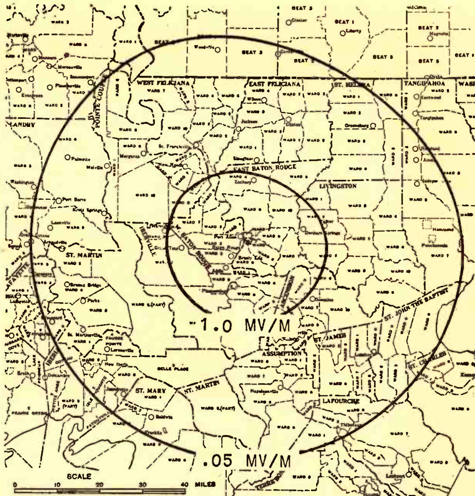
Fig. 5—A typical radio contour map, showing 1,000 and 500 microvolt-per-meter coverage.
